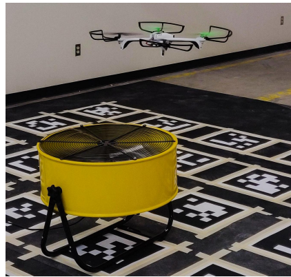
Fig. 1: The UAV is tasked to fly from Point A to Point B and back to A again. If the UAV flies over the fan while it is on, it crashes with high probability. Success or failure to return to the launching point provides information about the operation of the fan.
