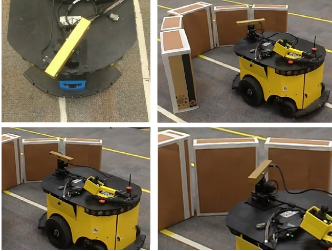
Figure 1 PowerBot by Adept MobileroBots capturing stereo observations during a navigation task
